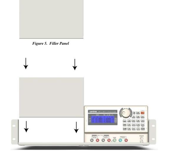
Figure 6. Filler Panel Placement
